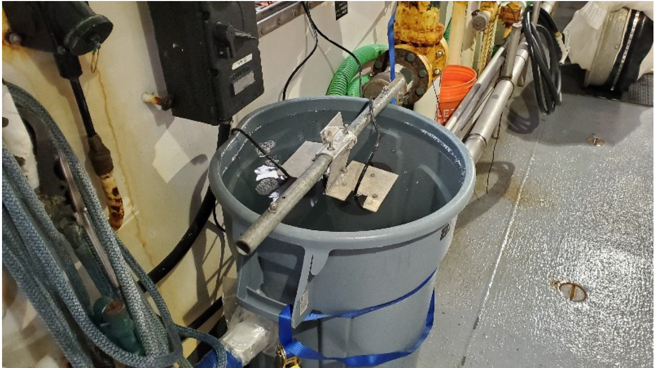
Figure 14. Animals were tethered in a 44 gallon aquarium with two transducers positioned in a bistatic setup.
